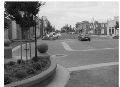
The improvements included creating pedestrian ramps that integrate carriage-height curbs and are ADA compliant; doubling available street parking by using diagonal stalls, resurfacing existing pavement; removing all aerial utilities and placing underground, installing landscaping with street trees; providing color coordinated street signs, benches, and vintage style street lighting, upgrading the storm drainage system, and water system.
